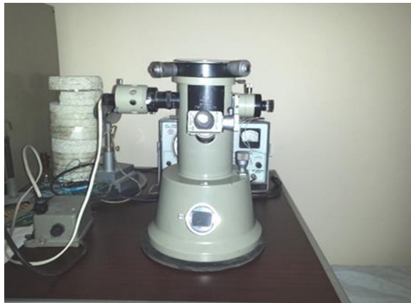
Fig. 3. Microinterferometer (MII-4) - measuring microscope with optical interference.
