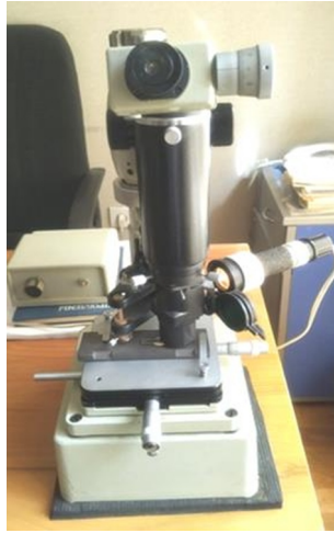
Fig. 4. Microhardness measuring microscope (PMT - 3).
